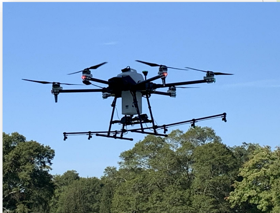
Drone specialized for crop input application
